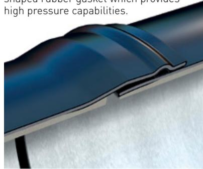
Full corrosion protection of the steel pipe is achieved by extending the Sintakote coating around both spigot and socket ends to underlap the cement mortar/calcium aluminate cement lining.
