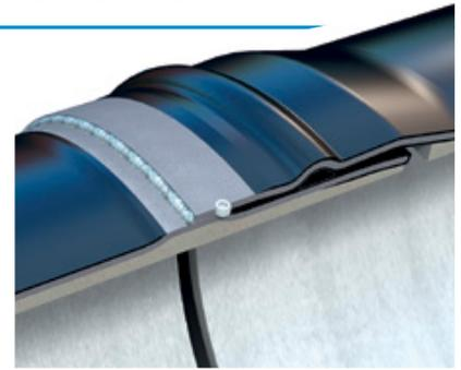
Steel Mains Sintalock joint consists of a rubber ring push-in joint and external site fillet weld. Sintalock does not require internal welding or CAC lining reinstatement and enables construction of a fully, end restrained pipeline without the need for concrete thrust blocks. This is a significant improvement on standard welded joints as it eliminates the safety issues associated with man entry as well as the need for joint reinstatement of the lining.
