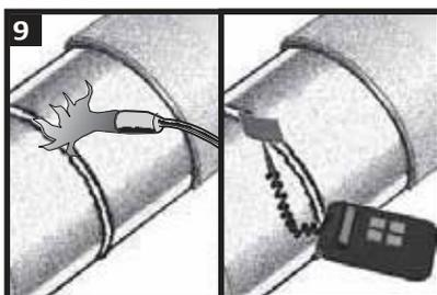
Pre-heat the joint area to 30°C or 3°C above ambient. Using a temperature measuring device, ensure that the correct temperature is reached on the steel and at least 50mm (2") on each side of the sleeve.
