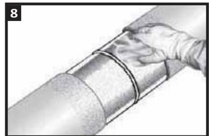
Wipe clean or airblast the steel and pipe coating to remove foreign contaminants.
