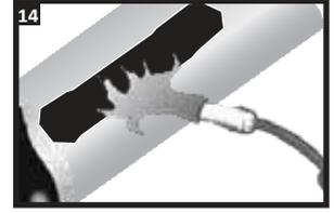
Gently heat the underside of closure patch to soften adhesive.
