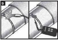
Pre-heat the joint area to 30°C or 3°C above ambient. Using a temperature measuring device, ensure that the correct temperature is reached on the steel and at least 50mm (2") on each side of the sleeve.
