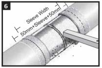
Ensure that the pipe is dry before cleaning. The steel joint area must be cleaned to a minimum of a wire brush finish. It is recommended to lightly abrade (with a hand tool) the pipe coating adjacent to the weld area to a distance of 50mm (2") beyond each end of the sleeve width.
