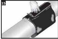
Centre the closure patch on the overlapping sleeve, press down firmly.
