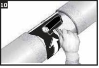
Coat the steel surface and 50mm on to the Sintakote at each side of joint with UCC Protek Butyl Multi Primer.
