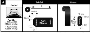
As a guideline, cut the required lengths of Sleeve material (L) and Closure material (W) from the bulk roll as follows
