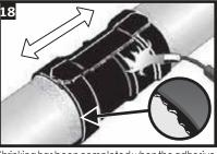
Shrinking has been completed when the adhesive begins to ooze at the sleeve edges all around the circumference. Finish shrinking the sleeve with long horizontal strokes over the entire surface to ensure a uniform bond.
